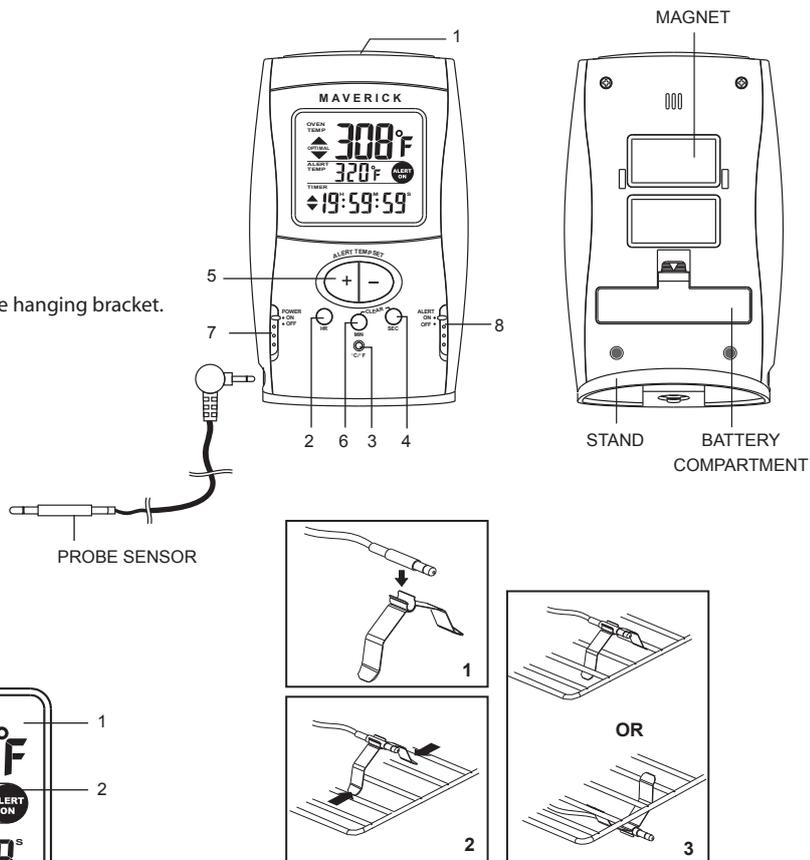
\* Make sure probe is properly mounted to the stainless steel clip and clip it to the wires of the rack inside your oven.
