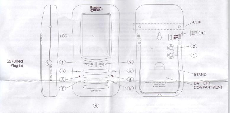
S2 (Direct Plug in) – allows you to plug 1 detachable stainless steel probe sensor directly into the receiver unit. LCD (Liquid Crystal Display) – Displays all icons, temperature and time. See LCD diagram for detailed information. CLIP – Removable clip allows you to be mobile. Clip the receiver unit to belt. BATTERY COMPARTMENT – Holds 2 AA batteries.
