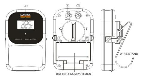
• LCD (Liquid Crystal Display) - displays temperature of both FOOD and BARBECUE. It will
